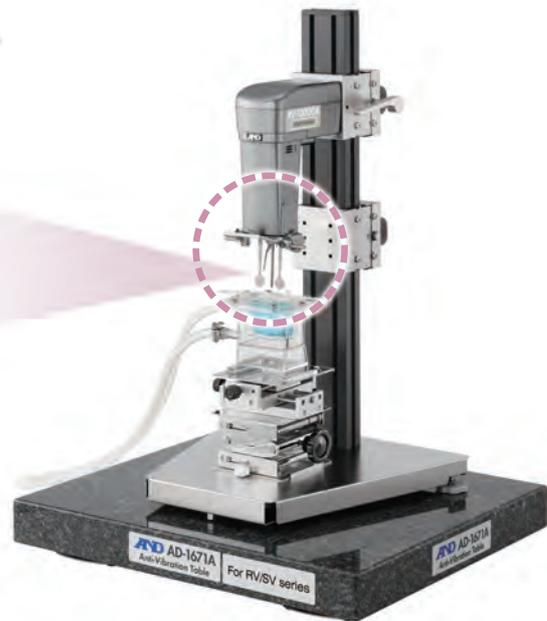
Two thin sensor plates in a tuning fork arrangement are driven with electromagnetic force to vibrate at their natural (resonant) frequency of 30 Hz within the sample fluid. Viscosity is then calculated based on the proportional relationship between the viscous resistance of the sample fluid and the amount of electric current required to drive and maintain the sensor plates at a constant vibration amplitude.\*<sup>1</sup> \*<sup>1</sup> Patented
