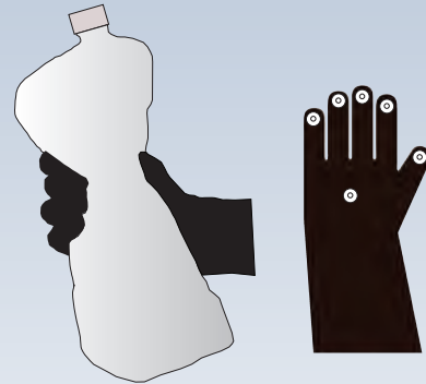
Measurement of force to crush plastic bottles
