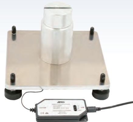
Measurement of grip strength to remove lids from jars
